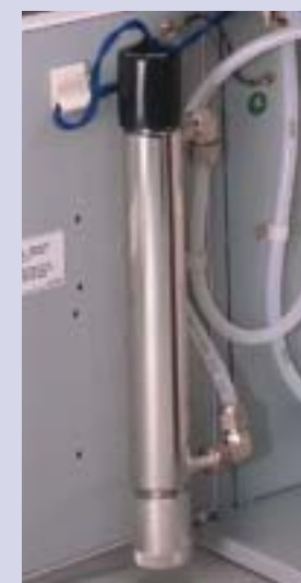
A dual wavelength UV lamp oxidizes organics to virtually undetectable levels and keeps bacteria to a minimum. The system displays an alert when the UV lamp should be changed.
