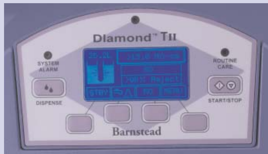
Digital display informs you of key information and alerts you when you need to maintain the system.
